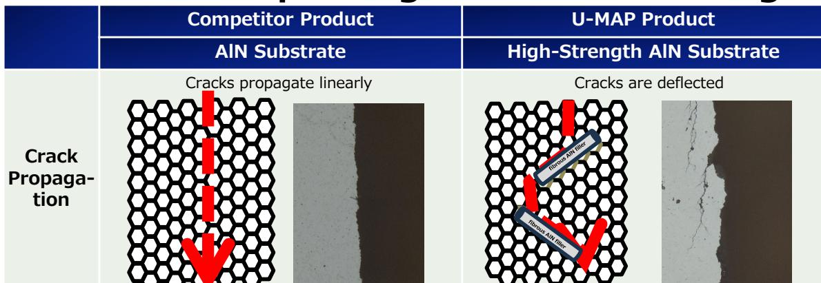
Fibrous AlN filler induces crack deflection, increasing fracture energy and thereby enhancing fracture toughness
