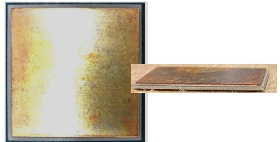
No cracking at 1500 cycles
